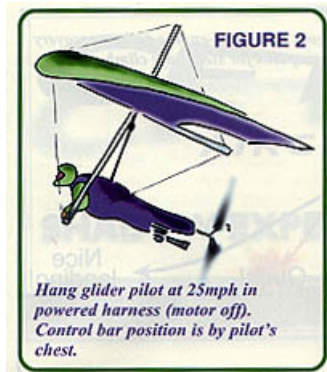
Hang glider pilot at 25mph in powered harness (motor off). Control bar position is by pilot's chest
