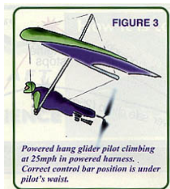
Powered hang glider pilot climbing at 25mph in powered harness. Correct control bar position is under pilot's waist
