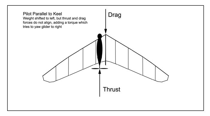
this in a lot of different ways, but the simplest one is to simply think of a twin-engine aircraft with the right engine dead - the thrust acting to the left of the centerline will tend to yaw the glider to the right, just the opposite of what we want.
