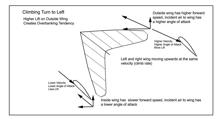
increases for the right/outer wing - so now the right wing has both a higher V and higher  $C_L(\alpha)$  than the left wing, and the roll moment becomes even larger. Thus we can expect to do more "high siding" to maintain a stable turn under power than we do when gliding.
