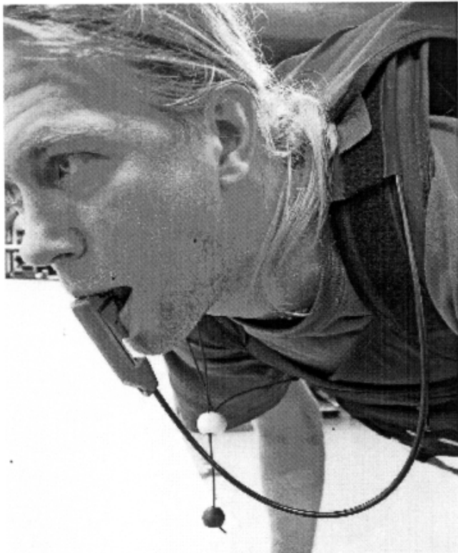
Mouth throttle. Strongly advised during take off and test running engine on ground.
