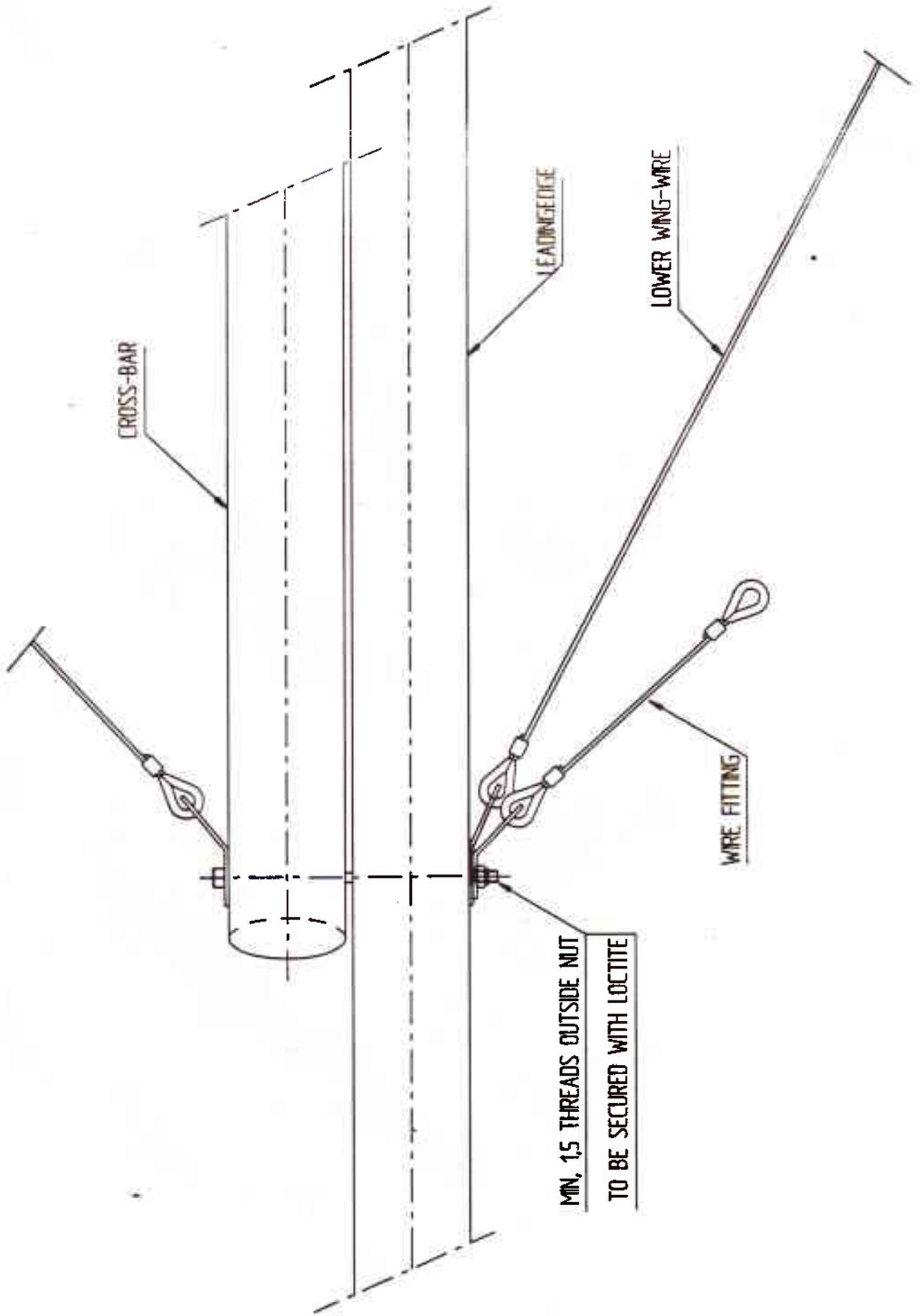
**FIG 3** Mounting of wire fitting.
